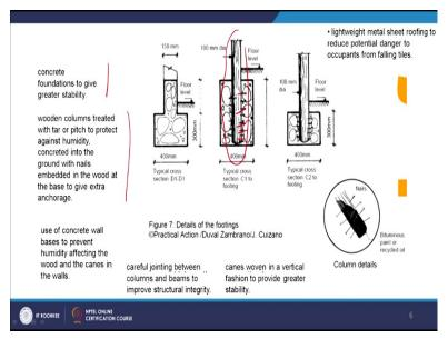
And what are the benefits of this quince constructions; one is they have upgraded this type of construction also embedded the concrete aspect and the concrete foundations. They provided the concrete foundations, so which can give more stability, greater stability towards the earthquake. Then, the wooden columns treated with tar or pitch to protect against humidity concreted into the ground with nails.
