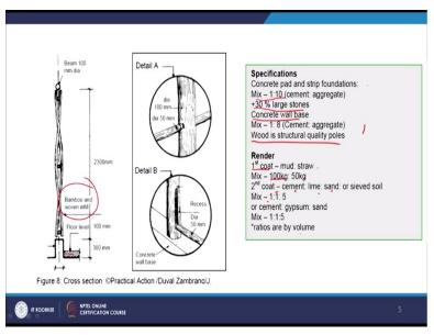
So, if you look at the cross-section of the woven timber, so this is how it looks where you have the floor level and about 300 mm height and then this woven timber is fixed upon it. So, this is about 2.3 meters, this is called we call it the woven infill and if you look at the detail A this junction and this junction, so these are the 2 junctions. So, now you have the 100 mm diameter and it has embedded the horizontal stud is embedded within it.
