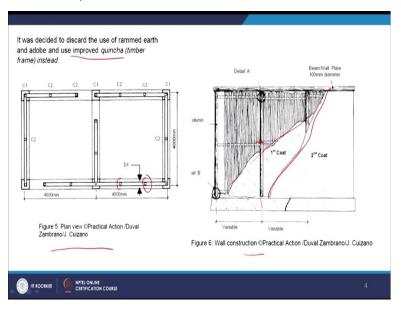
And they want to promote the quincha timber-frame instead to be as a better earthquake-resistant material. So, what you can see is from the practical action groups, the model they developed the plan with the timber posts in between and they have this is called quincha construction. So, what you can see here is it is a kind of timber studs embedded in the either in the concrete bedding or little deeper into the foundation.
